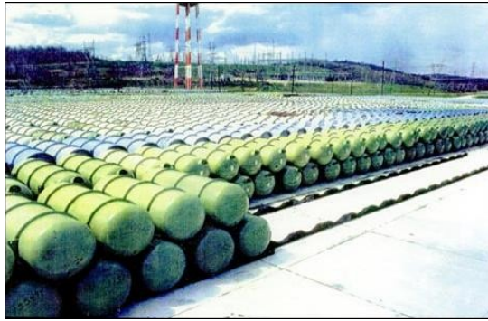
Steel cylinders of uranium hexafluoride in Piketon Ohio, currently awaiting deconversion and disposal
